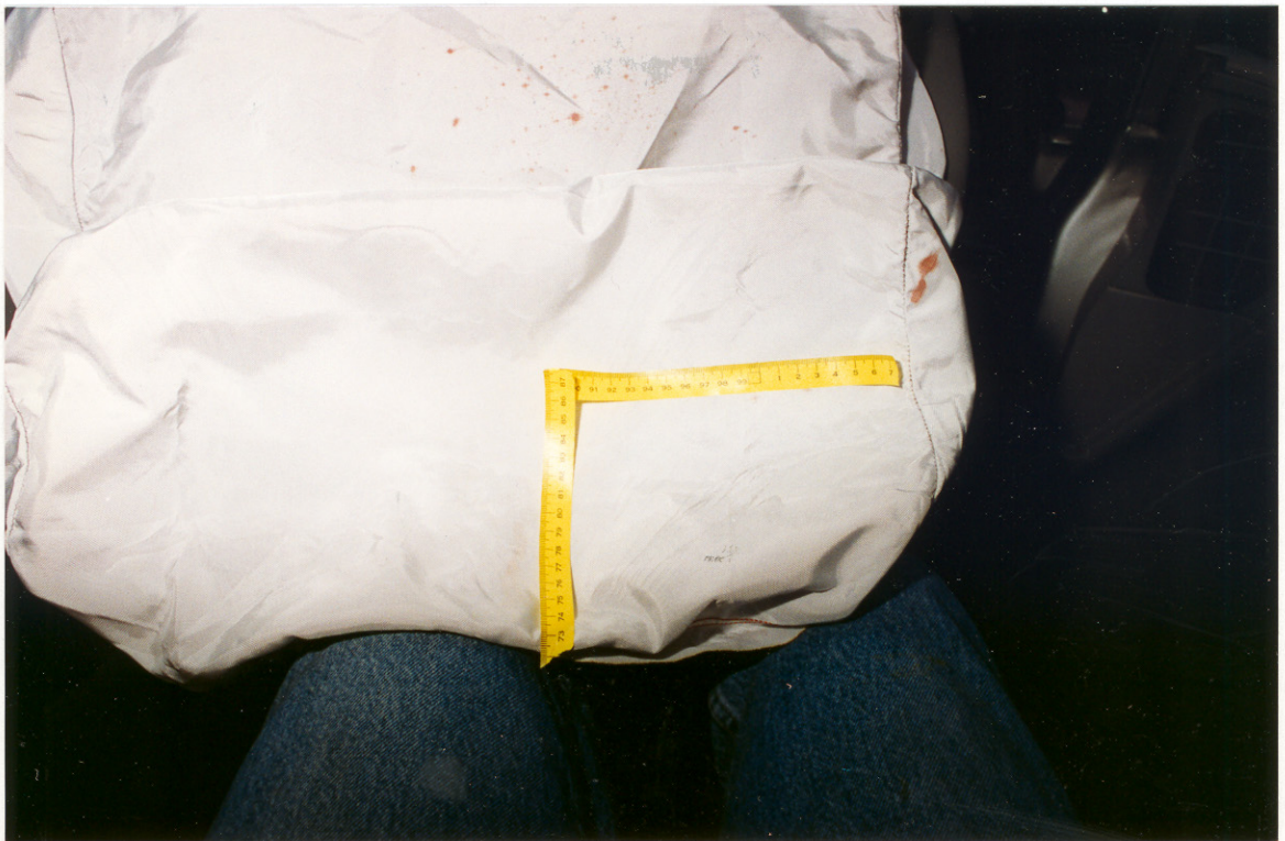
74. View of a gray vinyl transfer on the lower left quadrant of the air bag.
